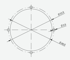
Dimension Tolerance DIN ISO 2768-m
