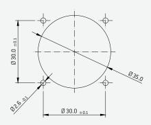
Dimension Tolerance DIN ISO 2768-m
